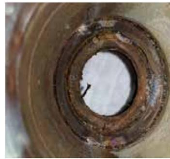
These are photos of the club's transfer pump which was returned to the club in a so called clean condition – note the oil seal is totally destroyed. This pump is a backup for our main bottling pump and therefore can no longer be borrowed by members.
