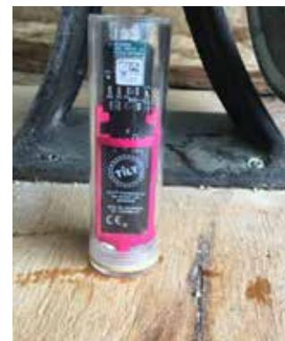
Hi tech - Floating hydrometer and thermometer
